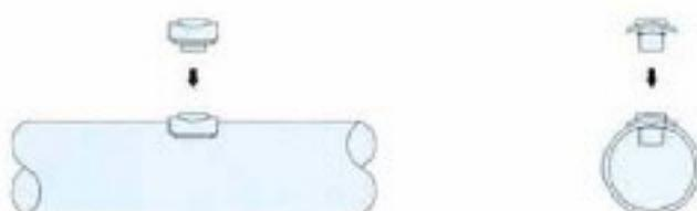
RCD-270 Step three: rotate and press RCD-270 in the PVC soft connector
